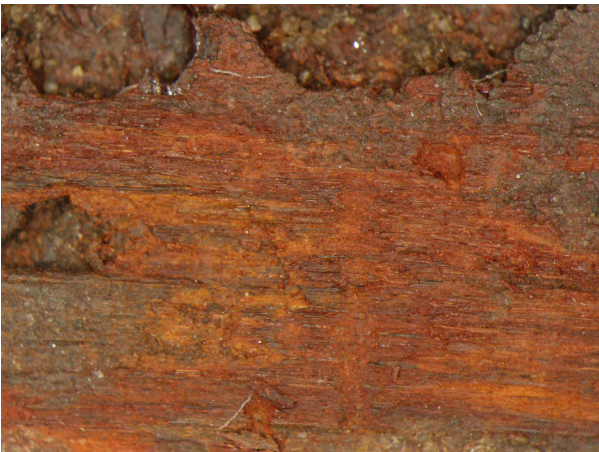
Fig. 10 - The wood traces are strongly fixed in the rust strata of the iron.
