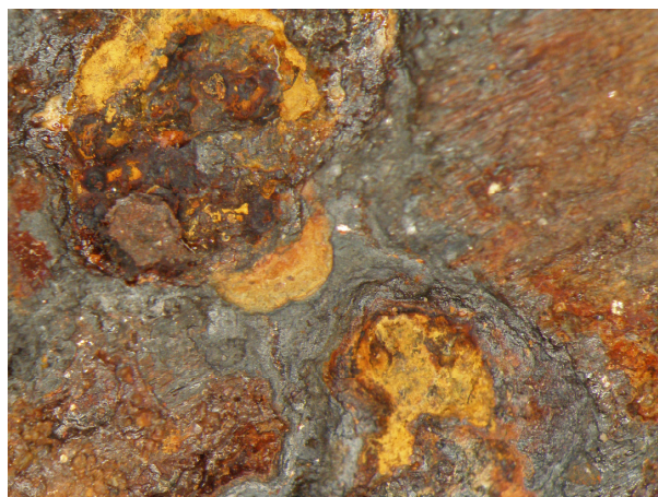
Fig. 15-16 - Ferrous or hidrated chlorides of white-yellowish to brown
