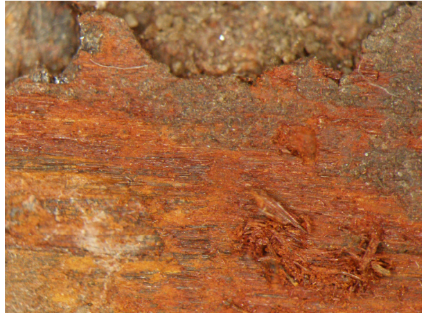
Fig. 11 - The wood is porous, pulverized, grinded.
