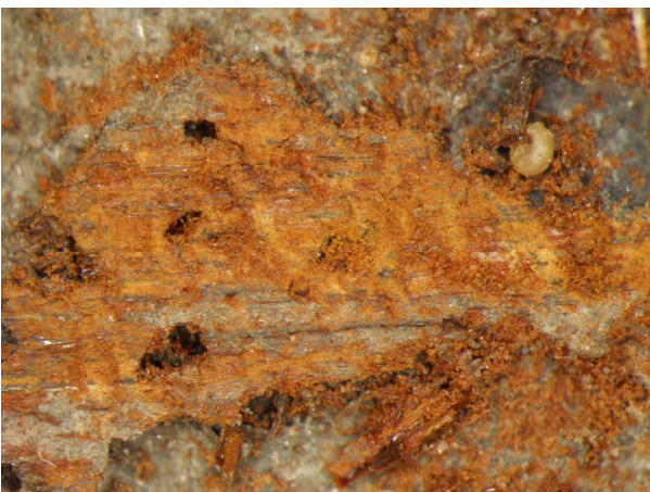
Figg. 12-13 - The biologic degradation caused by mushroom infestation over the wood.
